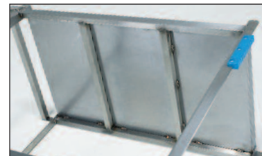
Shelves reinforced with square tubing.
